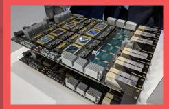
Announced at Computex, Taipai at the end of May, the world's most powerful cloud server platform for Al and HPC, NVIDIA HGX-2, was on display at ISC; the first time it has made an appearance in Europe. During ISC, there was a steady stream of attendees keen to see the SuperServer in real-life & photograph it. Similarly, to the NVIDIA DGX-2, this SuperServer also features 16 of the latest generation NVIDIA V100 GPUs.
