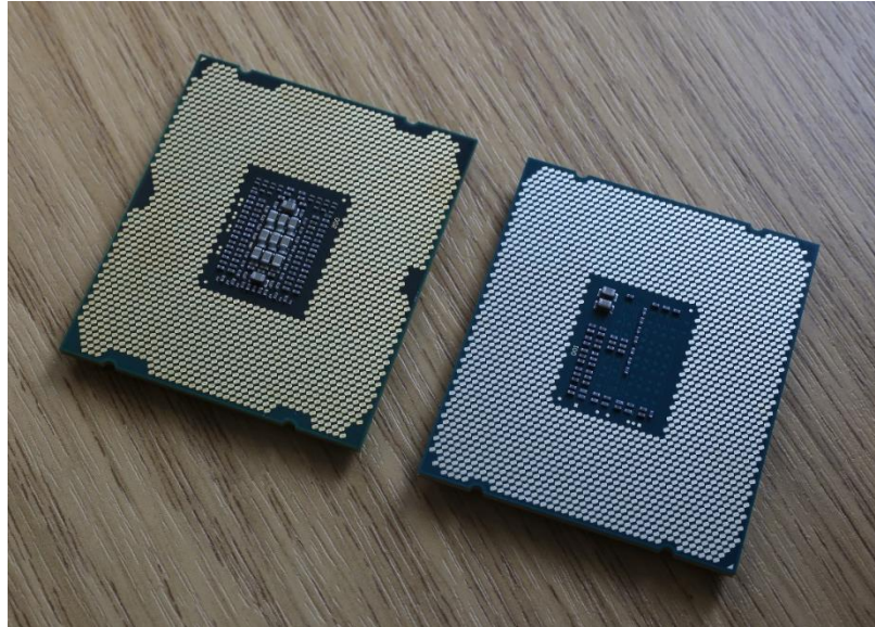
A Xeon E5-2600 v2 (left) pictured with the new Xeon E5-2600 v3 Series (right)
