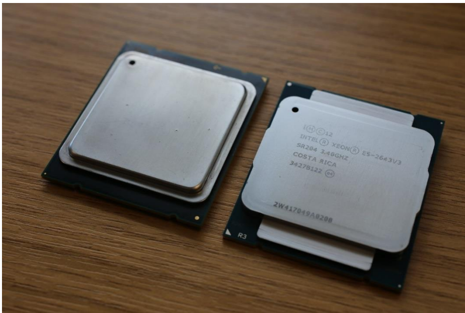
A Xeon E5-2600 v2 (left) pictured with the new Xeon E5-2600 v3 Series (right)
