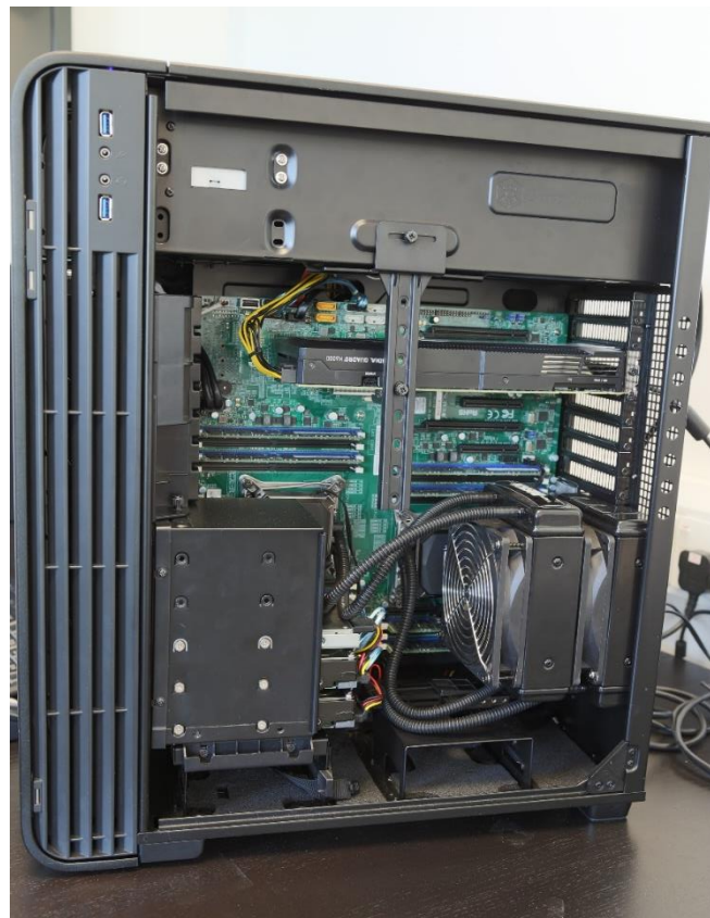
The Boston Venom 2401-12T and its liquid cooled E5-2687W v3 processors
