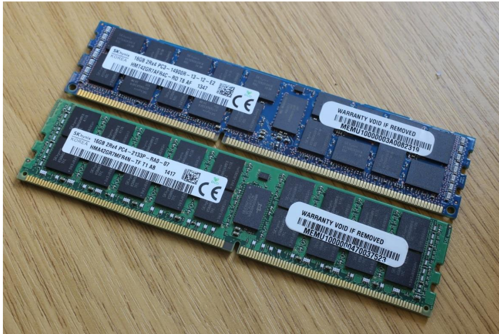
A DDR3 Module (top) compared to a DDR4 Module (below) Notice the elongated contacts in the centre
