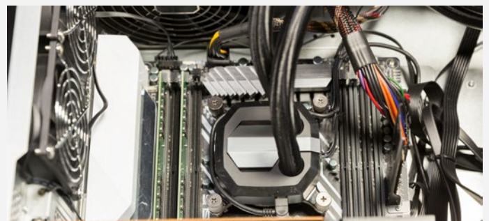
Image 2: A chill plate cooling a CPU in a gaming workstation with liquid pipes in and out of the plate.
